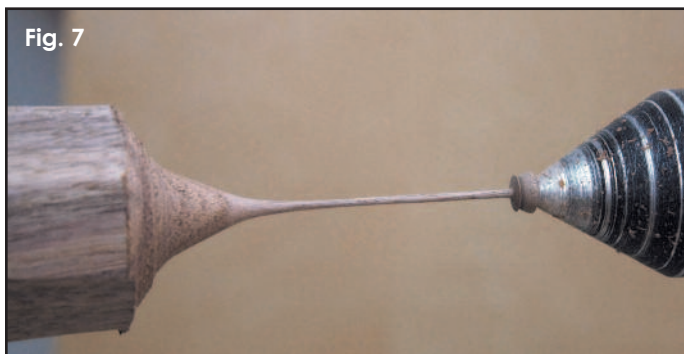
Fig. 7 The stem is about halfway turned.
