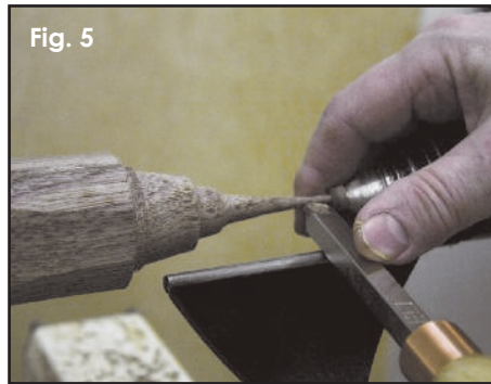
Fig. 5 Work down the taper with the easy finisher, supporting the tool behind the wood.
