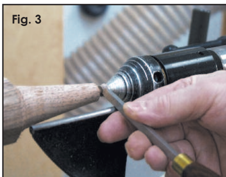
Shape the end cup with a small skew.
