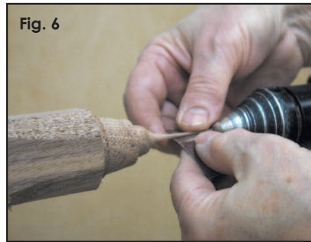
Fig. 6 Sand a completed section, supporting the stem to prevent flexing.
