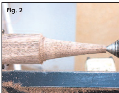
Turn the blank with the tapered cone at the end.
