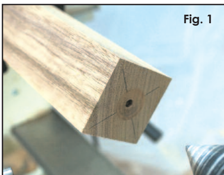
The blank is mounted with the hole and recess in the end.
